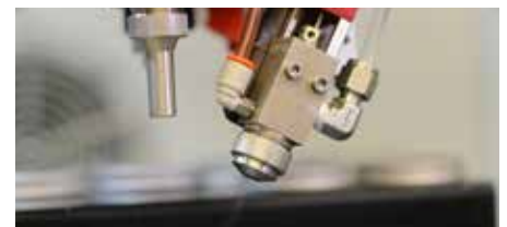
Spraying of the coating needs to be continuous for quality coverage.
